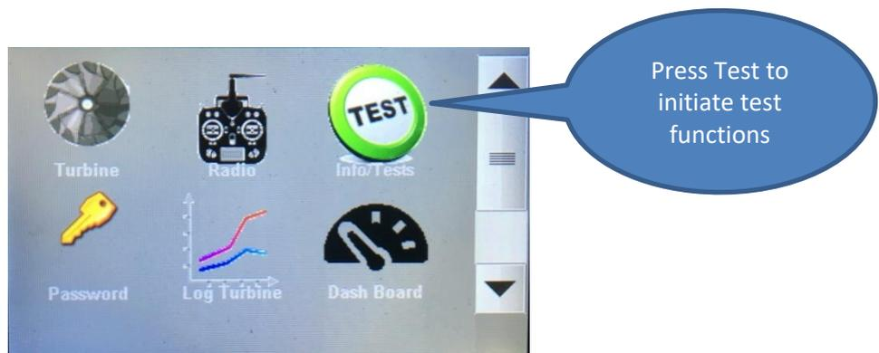
Test/Info page 1 displays Turbine Total Time in minutes, last Cycle time in seconds and number of cycles. Note: These numbers are reset to 0 upon overhaul. (Interval 25 hours)
