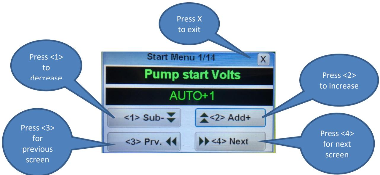
Pump start Value: Sets the power of the pump when it is started at the beginning of the fuel ramp.
