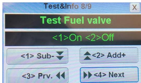
Test/Info page 9is used for priming the turbine.
