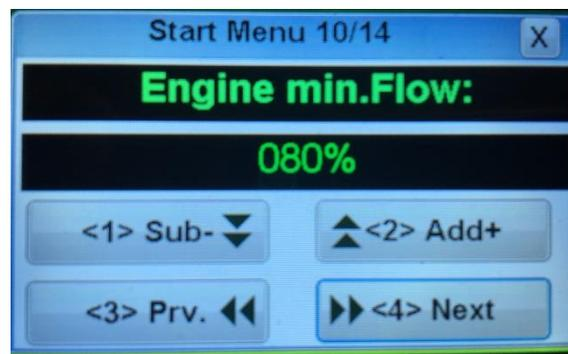
Stage 1 fuel duty: The percentage of total fuel applied during Stage 1 of startup.
