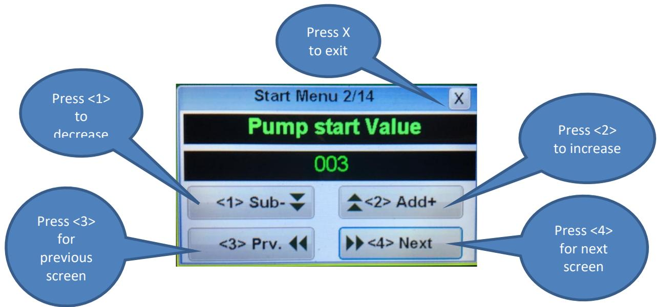
This parameter regulate the amount of fuel goes to the burner plug for an ignition. This parameter along with stage 1 fuel often need to reduced during winter months to avoid a flood none start. However, as the weather warms up, the original values need to be restored.
