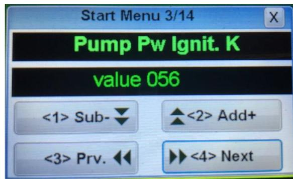
Ignition RPM: Sets the rpm where the starter will be switch off during ignition
