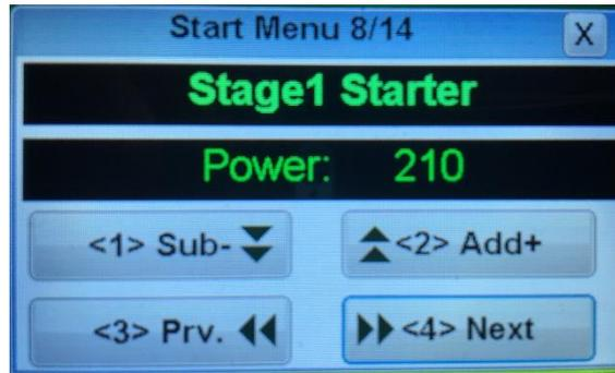
RPM 100% starter power: The resulting RPM value that is considered 100% maximum starter power.
