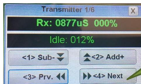
Note: The Correct reading of throttle % by the ECU can be verified on this screen, percentage of the throttle position is shown on, 0% in the position of engine stop (trim and stick down), 100% with stick/trim full up and between 10% and 30% at idle, (stick up trim down).
