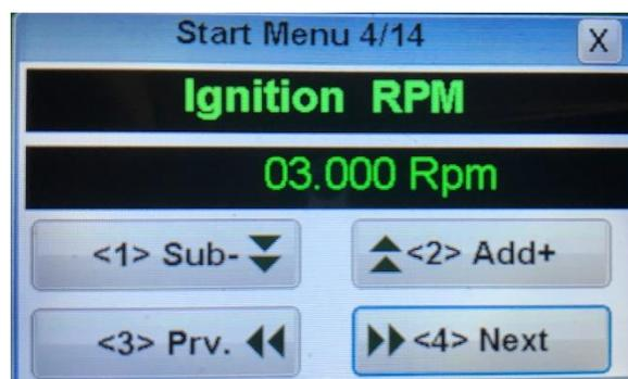
Stage 1 RPM: The RPM that triggers stage 1 of startup.
